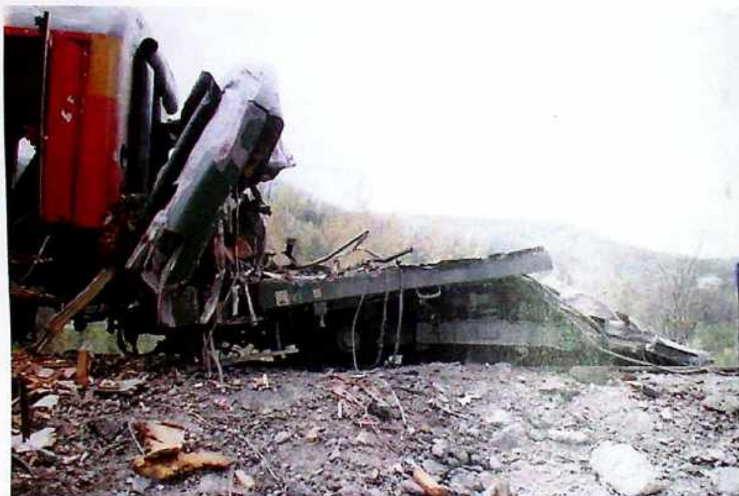
Photo 43 Close-up of the damaged and severed front part of the second carriage
