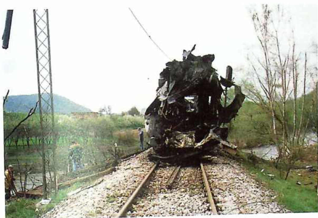
Photo 41 View and damage of the second carriage, including the severed part
