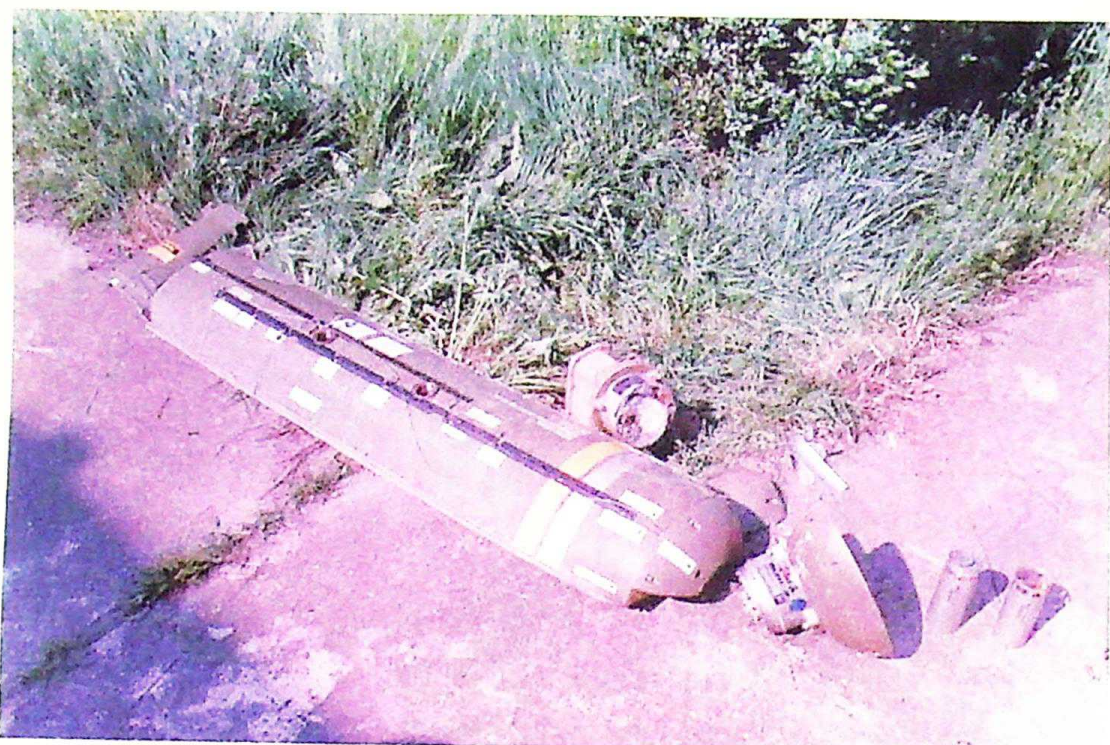
Photo 5 Fragments of a cluster bomb filled with carbon fiber reels
